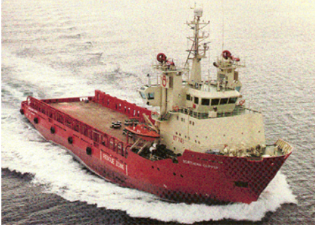
Fig. 1. Offshore supply vessel Northern Clipper of length L = 76.2 m.
