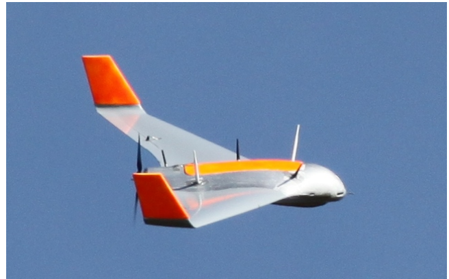
Figure 8. NTNU’s X8 flying-wing UAV used for flight tests.
