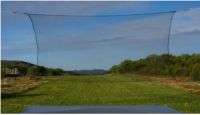
Figure 9. The recovery net used, approximate 5 x 3 meters.
