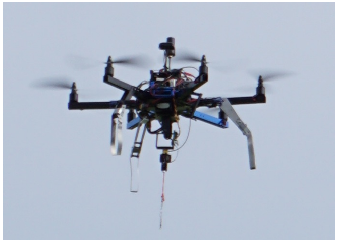
Fig. 1 Hexacopter type multirotor carrying a suspended load. The mechanism under the UAV body provides measurements of the deflection angle of the attachment wire.
